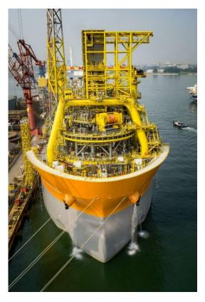
Figure 14 – The FPSO deployed for the case study project being prepared before arriving on location. The large yellow structure on the foredeck is the turret mooring system which connects the vessel to the 3000T disconnectable buoy.
