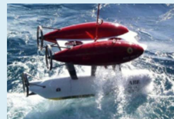
Autonomous Benthic Explorer ROV (Source: NOAA)
