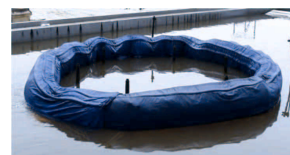
c. Water Cooling System Boom
