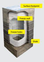
The recently completed Freeze Wall Test, located on Shell's private property in Rio Blanco County, Colorado, was a major, multi-year test of a commercial freeze wall prototype. The project successfully demonstrated that groundwater can be kept out of subsurface production areas using a frozen, underground barrier.
